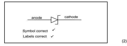
9.1.2 It has a very precise reverse breakdown voltage point. ✓
