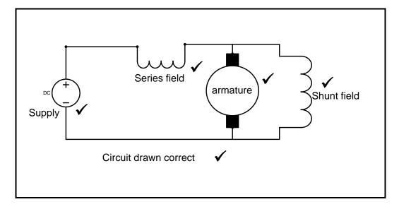
3.6 The speed stays virtually constant with an increase in load. ✓ It has the constant speed of shunt machines and the high starting torque of series machines. ✓
